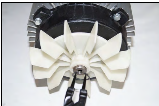
Remove lock ring from rotor shaft.
